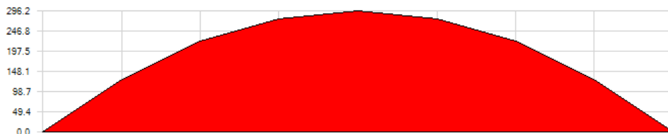
MOMENT DIAGRAM (k-ft) (Comb: 1.2D+1.6L+0.5S)
